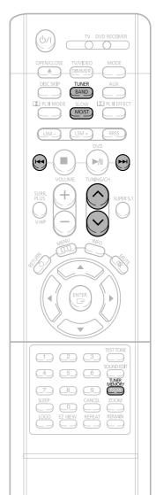
Press **MO/ST** button to listen in Mono/Stereo. (This applies only when listening to an FM station.)
